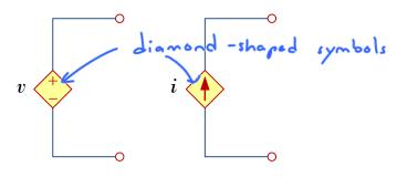
1.3.4. The key idea to keep in mind is that a voltage source comes with polarities (+ -) in its symbol, while a current source comes with an arrow, irrespective of what it depends on.
