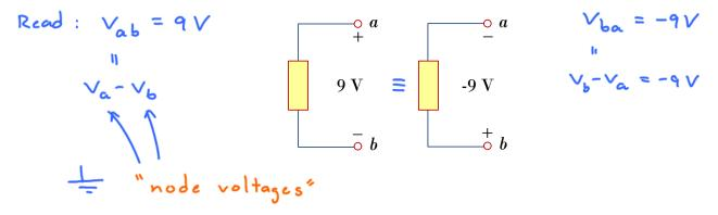
1.2.9. Like electric current, a constant voltage is called a **dc voltage** and is represented by V, whereas a **time-varying** voltage is represented by v. A time-varying voltage that is sinusoidal is called an **ac voltage**.
