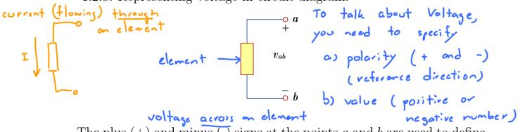
The plus (+) and minus (-) signs at the points a and b are used to define reference direction (voltage polarity).
